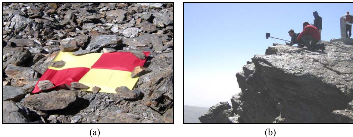
Figure 2. (a) Photogrammetric control point; (b) Photogrammetric shots from mount Veleta towards the rock glacier.
